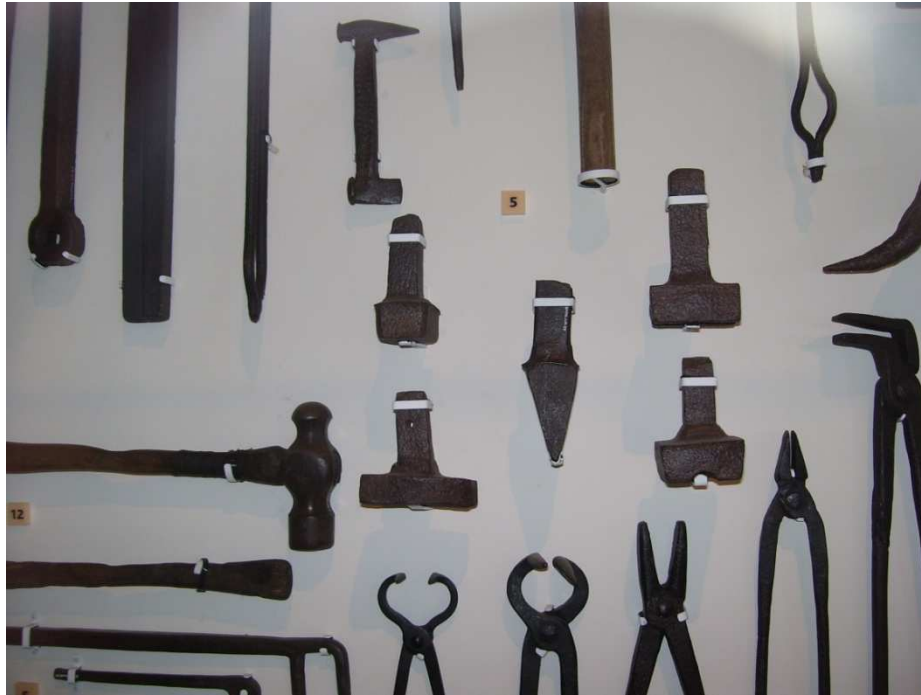
Centre group of small hardie hole tools, clockwise from top left: 1) Bottom swage tool. 2) Bottom swage long channel. 3) Bottom swage with narrow channel. 4) Bottom swage with broader channel. 5) in centre of group - Mandrel for the hardie hole.
